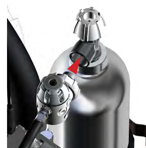
Figure 1-34. Align the oxygen regulator with the oxygen cylinder female DIN thread. Push it in and hand tighten the oxygen swivel nut.
