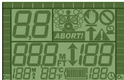
Figure 2-4. The Primary Display showing all LCD elements.
