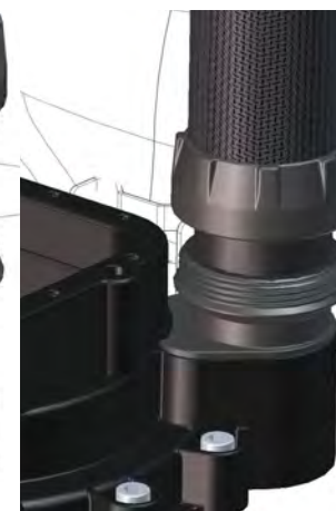
Figure 1-23. Push hose connector into receiver until outer flange is flush with start of threads.
