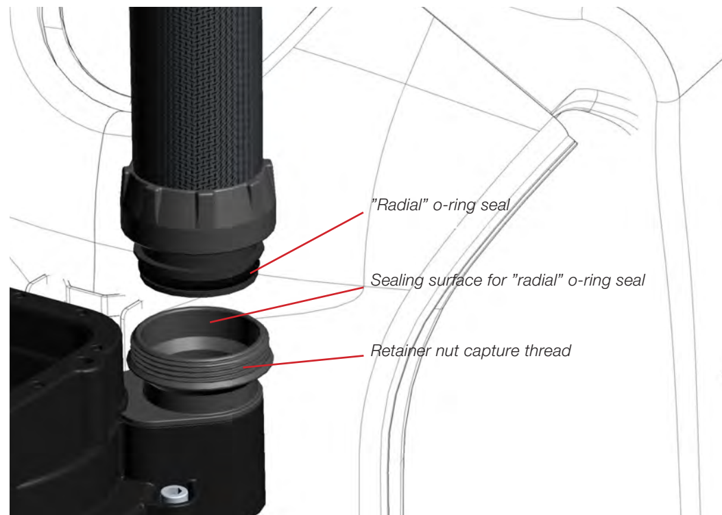
Figure 1-11. Typical “ Radial “ type o-ring seal.
