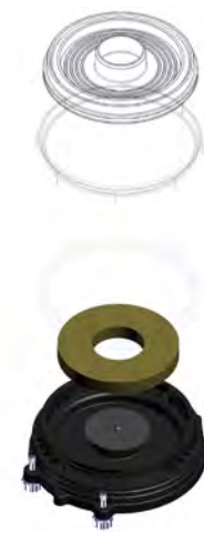
Figure 1-53. Lift and remove the lower sponge; inspect for collected water. Rinse, dry, and store the lower sponge; disinfect if desired.
