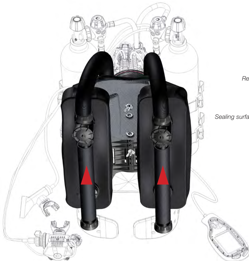
Figure 1-42. Breathing hoses properly connected onto the water diversion manifolds.
