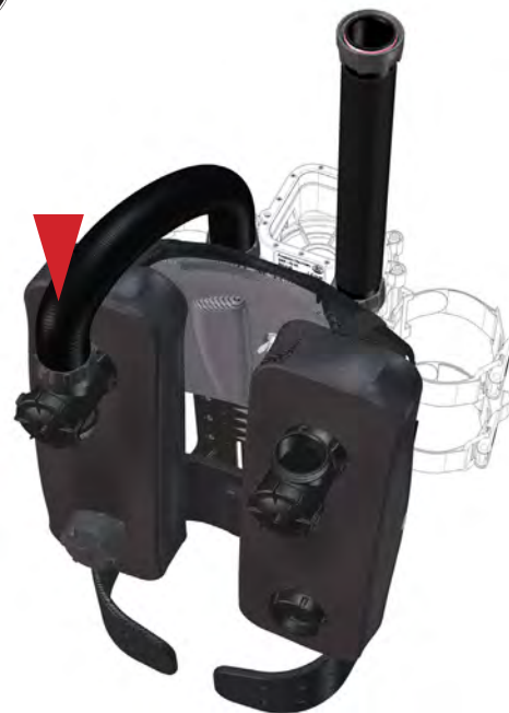
Figure 1-25. Attach the right counterlung water diversion manifold to the right rear breathing hose.
