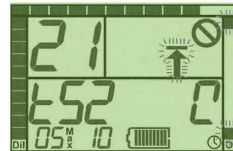
Figure A2-9: Oxygen confirmation screens at test 52, showing the alternating values of "O 2 " (for "Oxygen"; top), "Fr" (for "Fraction"; middle), and a numeric value (indicating the assumed fraction of Oxygen; bottom) for the diluent mixture.
