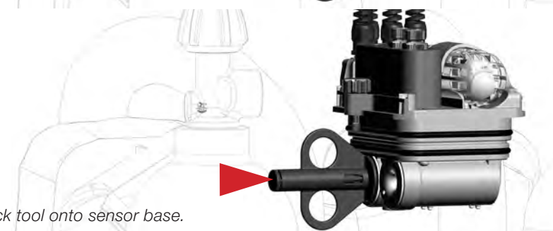
Figure 4-2. Removal tool snapped into sensor base.
