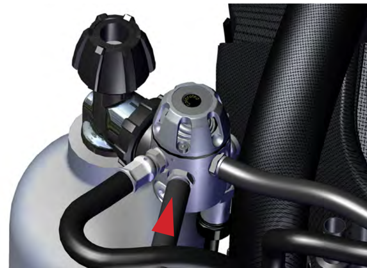
Figure 1-41. Connect the alternative air source low pressure hose to a low pressure port (marked "IP") on the diluent (black connection wheel) 1st stage.
