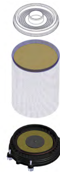
Figure 1-52. Remove the end plate.
