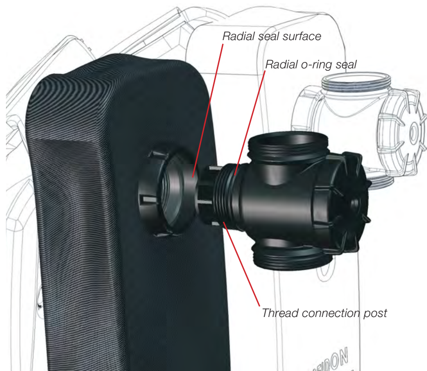
Figure 1-17. Insert the right hand water diversion manifold into the port on the right counterlung.
