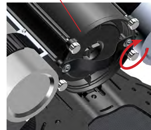
Figure 1-62. Tighten the four screws.
