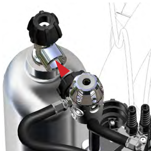
Figure 1-33. Align the diluent regulator with the diluent cylinder female DIN thread. Push it in and hand tighten the diluent regulator swivel nut.
