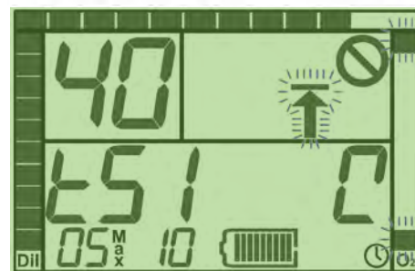
Figure A2-3: Helium confirmation screens at test 51, showing the alternating values of "HE" (for "Helium"; top), "Fr" (for "Fraction"; middle), and a numeric value (indicating the assumed fraction of Helium; bottom) for the diluent mixture.
