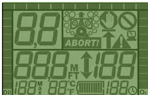
Figure 2-4. The Primary Display showing all LCD elements.
